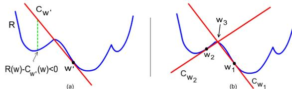
Figure 1. Cutting planes and linearization errors
