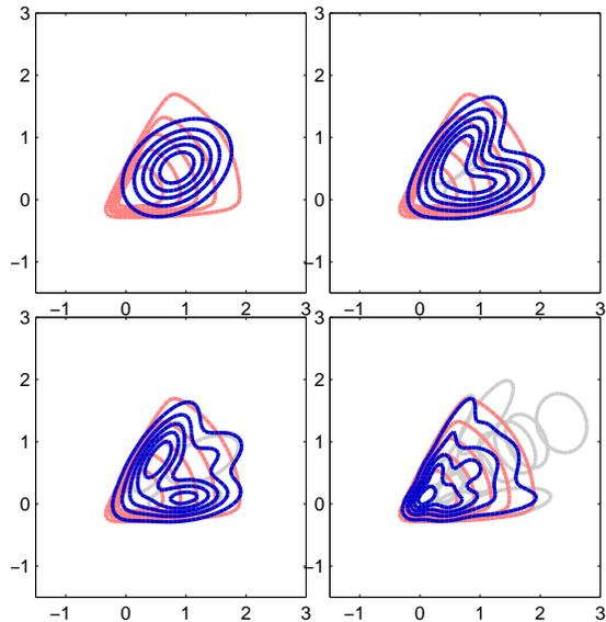
Figure 4. A 2D example of split Mean-Field for  $f(x) = \mathcal{N}(x)\sigma(20x_1 + 4)\sigma(20x_2 - 10x_1 + 4)$ . The true function is given by light contours, the mixture approximation by dark contours and the individual Gaussian components by light elliptic contours. Iterations 1, 2, 3 and 300 are shown. There were 14 components at the 300th iteration.
