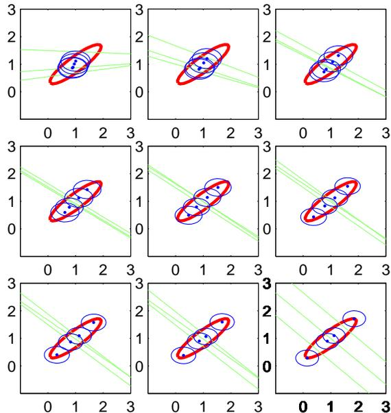
Figure 2. First 9 iterations of the 4-components split mean field algorithm. The red ellipse is the true function. The blue circles are the factored distribution approximating it. The green lines represent the component splits.
