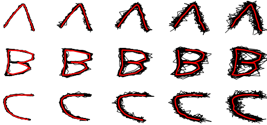
Figure 8. In bold, trajectory retrieved by a model trained successively with a dataset containing (from left to right) r^s = \{10\%, 20\%, 30\%, 40\%, 50\%\} of noise, using PCA decomposition.
